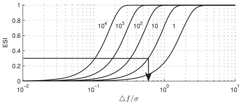
Figure 3: Expected SI for the  $N$ -spike criterion with ideal memory as a function of  $\Delta f/\sigma$  for various  $N$ . For  $N \in \{1, 10\}$ , the curves were computed using equation 4.11; for  $N \in \{100, 1000, 10,000\}$ , the curves were computed using equation 4.12. The arrow reads off the  $N = 10$  curve the ratio  $\Delta f/\sigma$  required to obtain an ESI of 0.31—the value obtained by Malmierca et al. (2009) for  $\Delta f = 0.15$  octaves (see text).
