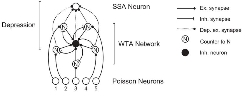
Figure 7: Diagram of a five-input abstract SSA model that implements the  $N$ -spike and depressing-standard criteria. The winner-take-all (WTA) section of the network implements the  $N$ -spike criterion and is responsible for estimating the incoming tone ( $\hat{X}$ ). The section labeled “depression” implements the depressing-standard criterion.
