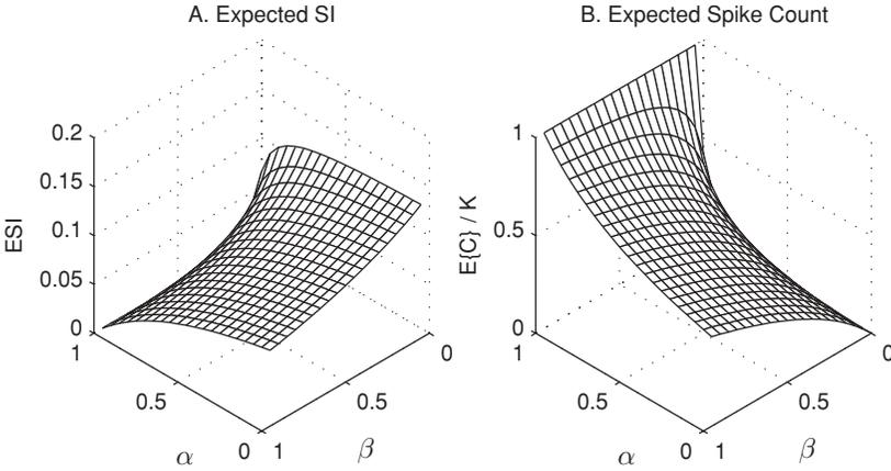
Figure 5: Surfaces plotting the (A) expected SI and (B) expected spike count ( $E\{C\}$ ) for various choices of adaptation ( $\alpha$ ) and recovery ( $\beta$ ) parameters, with  $\Delta f/\sigma = 0.60$ ,  $p_{dev} = 0.1$  and  $N = 10$ . The ESI for an ideal memory is 0.3075.
