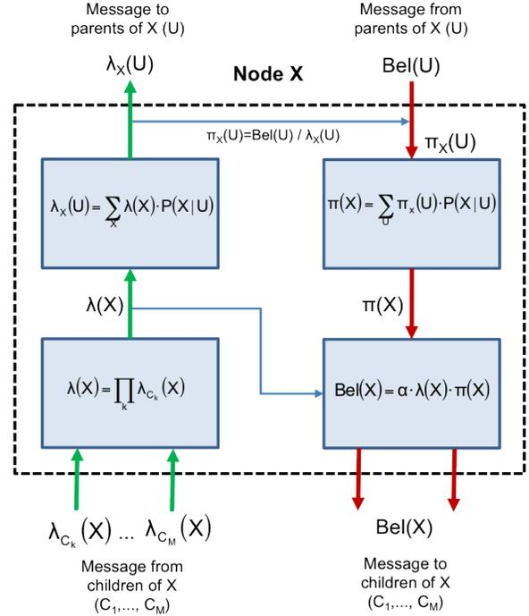
Fig. 1. Internal structure of a Bayesian node implementing belief propagation
