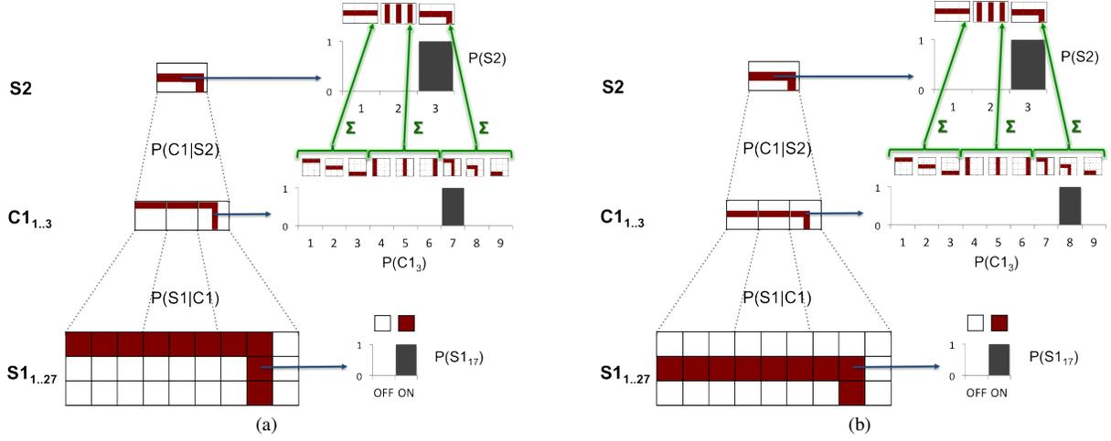
Fig. 2. Bayesian network that approximates the selectivity and invariance operations using belief propagation. This example illustrates how grouping C1 states achieves translation invariance. The S1 and C1 representation in a) and b) differ in the location of their pattern, but the S2 representation is invariant to position and, thus, equivalent in both cases.
